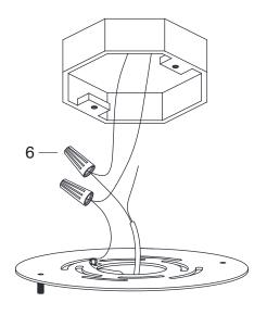
**5** Connect the fixture black wire to the hot wire in the junction box using the wire nut (6).
