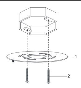
2 Attach the mounting plate (1) to the junction box with the mounting screws (2) provided.
